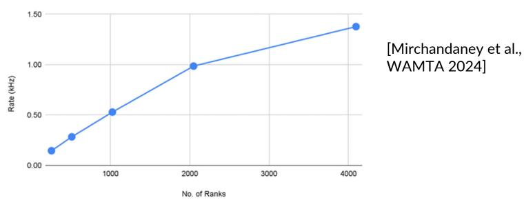
Weak scaling on up to 4096 GPUs on Frontier
